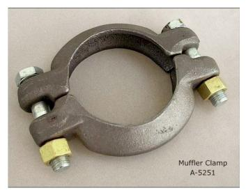
Now apply the clamp, I usually have the bolts already on the rear clamp, then once the rear clamp is in place, fit the front clamp and apply the nuts. Tighten these nuts, and let the sealer dry overnight for best results. After the first start up and heat up, let everything cool, then re-tighten the nuts.
